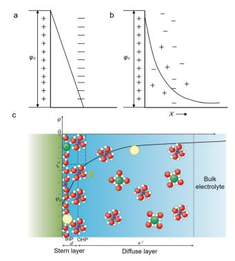
Fig. 1 Schematic description of different EDL models at a negatively charged electrode. (a) The Helmholtz model. (b) The Gouy-Chapman model. (c) The Gouy-Chapman-Stern model. 40 The yellow, green, purple, red, and white spheres represent neutral species, the anions, the cations, oxygen and hydrogen. Reproduced from ref. 40 with permission from the Springer Nature, copyright 2021.
