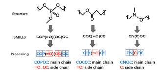
Fig. 7 The process of converting polymer structures to SMILES strings and further preparation to generate input descriptors for machine learning models. Reproduced from ref. 109 with permission from the Royal Society of Chemistry, copyright 2021.
