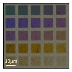
Fig. 6 Bright-field optical microscopy image of Mie resonators characterized by (L.g) geometric parameters in the range L(60 nm-100 nm) and g(60 nm-100 nm).
