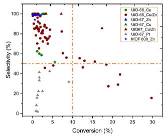
Fig. 10 Selectivity toward methanol versus conversion of CO<sub>2</sub>. While different symbols represent various metal-organic frameworks, different colours represent various incorporated metal active sites. 37-46 Orange dashed lines represent 10% conversion and 50% selectivity and have been included to guide the eyes.
