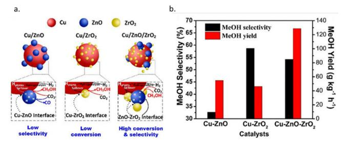
Fig. 5 (a) Schematic diagram of the  $CO_2$  hydrogenation process over Cu-ZnO,  $Cu-ZrO_2$  and  $Cu-ZnO-ZrO_2$  catalysts. (b) Methanol yields and methanol selectivity of Cu-ZnO,  $Cu-ZrO_2$  and  $Cu-ZnO-ZrO_2$  catalysts. Reprinted with permission from ref. 78. Copyright 2019 American Chemical Society (https://pubs.acs.org/doi/full/10.1021/acscatal.9b01943).
