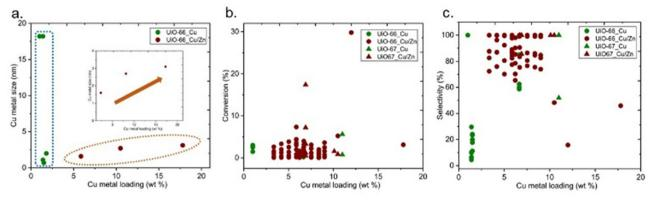
Fig. 14 (a) Cu metal size *versus* Cu metal loading (b) conversion of CO<sub>2</sub> *versus* Cu metal loading (b) selectivity towards methanol *versus* Cu metal loading.
