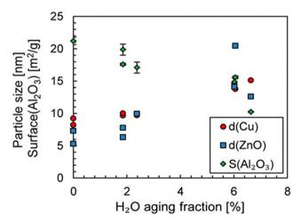
Fig. 6 Influence of H<sub>2</sub>O volume fraction on the Cu and ZnO particle size and  $Al_2O_3$  surface. The aging period was 48 hours. Reprinted with permission from ref. 85. Copyright 2019 American Chemical Society (https://pubs.acs.org/doi/full/10.1021/acs.iecr.9b01898)
