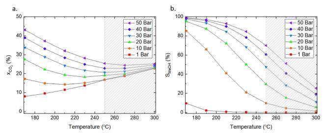
Fig. 2 Influence of pressure and temperature on (a) equilibrium conversion of CO<sub>2</sub> and (b) selectivity toward methanol at equilibrium. The dashed area indicates the temperature range typically applied for  $CO_2$  hydrogenation to methanol in industry. The ratio of  $H_2/CO_2$  was 3:1, and methane was excluded from the calculations. Factsage was used for the analyses.<sup>55</sup>
