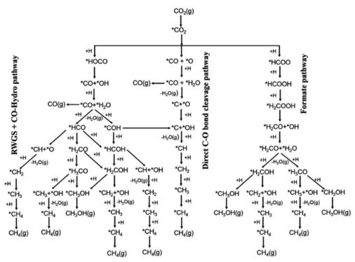
Fig. 3 Possible reaction pathways of CO<sub>2</sub> hydrogenation to CO, CH<sub>3</sub>OH, and CH<sub>4</sub>. \*(X) indicates adsorbed species. Reprinted with permission from ref. 57. Copyright 2017 American Chemical Society (https://pubs.acs.org/doi/10.1021/jacs.7b05362).
