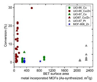
Catalytic conversion versus BET surface area of metal incorporated Fia. 9 MOFs.
