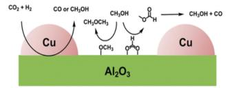
Fig. 4  $CO_2$  hydrogenation on  $Cu/Al_2O_3$ . Used with permission of Angewandte Chemie International Edition, from  $CO_2$  Hydrogenation on  $Cu/Al_2O_3$ : role of the metal/support interface in driving activity and selectivity of a Bifunctional Catalyst, Lam *et al.*, 2019, **58**, 39 permission conveyed through Copyright Clearance Center, Inc.
