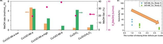
Fig. 11 (a) Rates of methanol (MeOH) production (orange bars), methanol selectivity (green bars) on selected catalysts at 250 °C and 32 bar, and activation energy (Ea, pink points). Reproduced from ref. 43 (https://www.nature.com/articles/s41467-020-19438-w) with the permission of unrestricted use (https://creativecommons.org/licenses/by/4.0/). (b) Selectivity toward methanol versus the number of missing linker defects per cluster. 40,43
