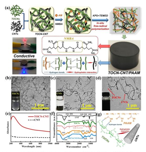
Fig. 2 (a) Synthesis process of the TOCN-CNT/PAAM hydrogels. TEM figures of (b) TOCNs, (c) CNT, and (d) TOCN-CNT nanocomposites. (e) UVvis data of CNT and TOCN-CNT. (f) FTIR data of TOCN-CNT/PAAM hydrogel and the components. (g) Illustration of the interactions among PAAM, TOCNs, and CNTs.38
