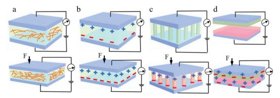
Fig. 8 Schematic illustrations of the four transduction mechanisms. (a) Piezoresistive. (b) Capacitive. (c) Piezoelectric. (d) Triboelectric. (106 Triboelectric. (107 Triboelectric. (107
