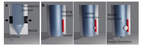
Fig. 15 Drop formation in piezoelectric (a) and thermal (b) inkjet systems. 192
