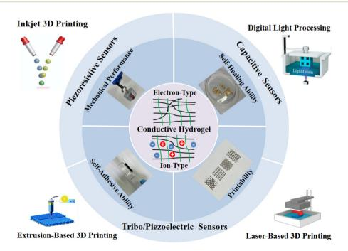
Fig. 1 Classification and properties of conductive hydrogels and the related 3D printing techniques.
