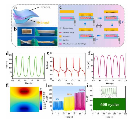
Fig. 11 (a) Structure of PP-TENG. (b) Images of PP-TENG under the different states. (c) Illustration of the power generation mechanism. (d) V<sub>OC</sub>, (e)  $I_{SC}$ , and (f)  $Q_{SC}$  of the PP-TENG. (g) Finite element analysis of PP-TENG output voltage. (h) Open-circuit voltage of the stretchable PP-TENG at different strains. (i) Stability of the PP-TENG under 600 cycles. 139
