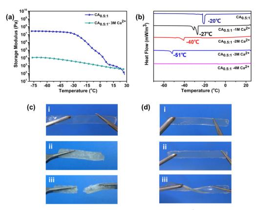
Fig. 5 Antifreezing test of ionic conductive hydrogel. (a) DMA curves of  $CA_{0.5:1}$  and  $CA_{0.5:1}$ -3 M  $Ca^{2+}$  when the temperature changes from 25 to -75 °C, (b) DSC curves of  $CA_{0.5:1}$  and  $CA_{0.5:1}$ - $Ca^{2+}$  when the temperature changes from 25 to -75 °C, and (c and d) images of  $CA_{0.5:1}$  and  $CA_{0.5:1}$ -3 M  $Ca^{2+}$  bending at -50 °C, respectively.<sup>77</sup>
