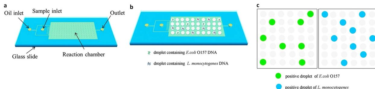
**Fig. 10** Droplet digital PCR workflow for simultaneous detection of *E. coli* O157 and *L. monocytogenes*. (a) Fabrication of mineral oil saturated PDMS (OSP) microfluidic chip. (b) Generation of droplets. (c) On-chip amplification under many times of thermal cycles followed by fluorescence readout. Copyright 2015 by Elsevier.<sup>126</sup>
