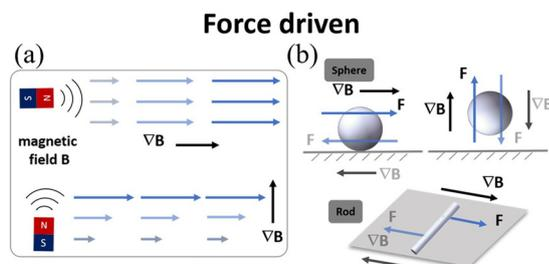
Fig. 8 (a) Schematic of magnetic field gradient actuation. (b) The typical models of magnetic field gradient-driven microrobots (sphere and rod).
