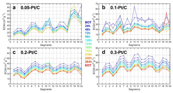
Fig. 3 Local ECSA along the gas channel measured in a segmented cell for CLs (a) 0.05-Pt/C; (b) 0.1-Pt/C; (c) 0.2-Pt/C and (d) 0.3-Pt/C. Segment #1 corresponds to the air inlet at the cathode and  $H_2$  outlet at the anode, while segment #20 corresponds to the air outlet at the cathode and  $H_2$ inlet at the anode.
