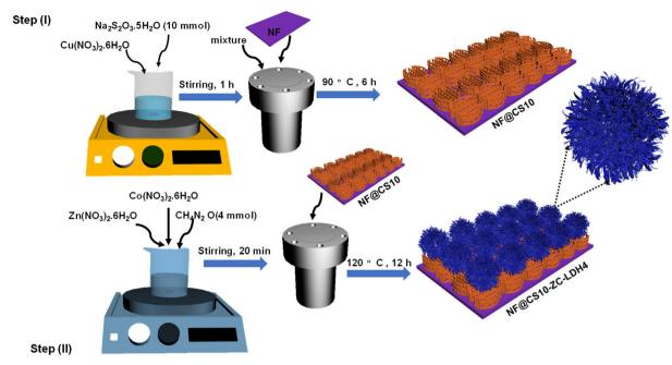
Fig. 1 Step (I) schematic diagram for the preparation of NF@CS10 nanosheets. Step (II) schematic diagram for the preparation of NF@CS10-ZC-LDH4.
