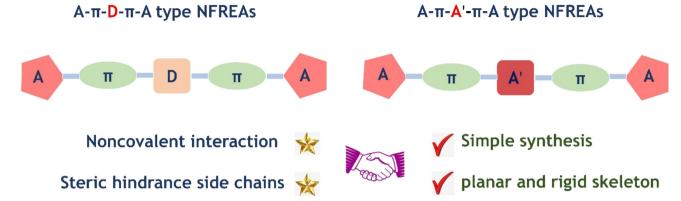
Fig. 1 Illustration of A- $\pi$ -D- $\pi$ -A or A- $\pi$ -A type NFREAs and the corresponding design strategies.
