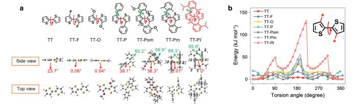
Fig. 8 (a) Chemical structures and DFT calculation results; (b) torsional energy profiles between two thiophenes for several bithiophene units (reprinted with permission from ref. 28 Copyright 2021 Springer Nature).
