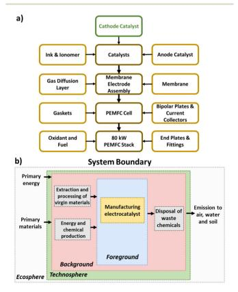
Fig. 1 (a) PEMFC stack component hierarchy, with highlighted focus on the cathode catalyst. (b) System boundary of the PEMFC cathode electrocatalyst LCA.
