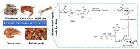
Fig. 6 The electrochemical scheme of chitin/NAG into acetate with a yield of over 90% in value-added electrolysis (a reaction pathway that produces acetate as the main product)
