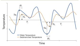
Fig. 5 Local max/min method scheme (based on Luce *et al.*, 2013). Definition for time differences ( $\Delta t_1$  and  $\Delta t_2$ ) and temperature ratios ( $Ts_1/Tw_1$  and  $Ts_2/Tw_2$ ) between local maxima and minima. Note that the sketch for the daily mean temperatures was simplified as these values might not coincide for liquid and sediment-bed time series.
