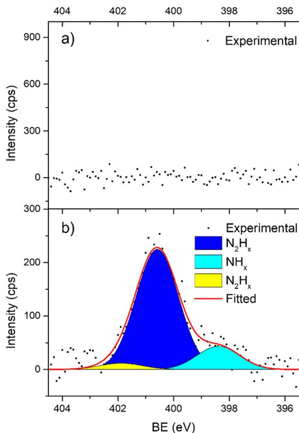
Fig. 9 High resolution N 1s spectra of Ir/graphite: (a) fresh and (b) used for 5 runs.
