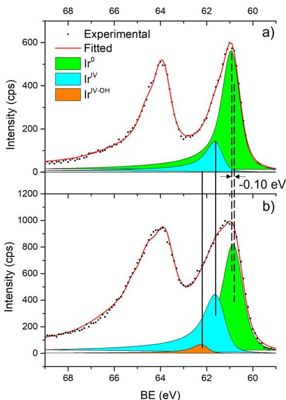
Fig. 7 High resolution Ir 4f spectra of fresh samples, (a) Ir/graphite and (b) Ir/GCN. For clarity, the comparison of the fitted contributions is limited to the Ir<sub>7/2</sub> components without any satellite.
