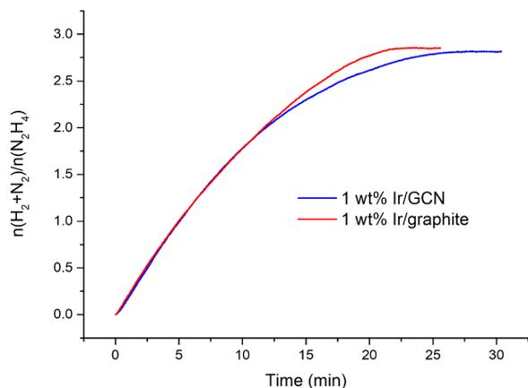
**Fig. 1** Kinetic profiles of 1 wt% Ir/graphite (red) and 1 wt% Ir/GCN (blue) catalysts for hydrazine decomposition. All tests were performed at 323 K and 1400 rpm, using 300  $\mu\text{L}$  of a hydrazine solution 3.3 M in 5 mL of NaOH 0.5 M and a  $\text{N}_2\text{H}_4 \cdot \text{H}_2\text{O}$ : catalyst molar ratio of 1000 : 1. A sampling time of 0.3 s was employed to obtain continuous kinetic profiles.
