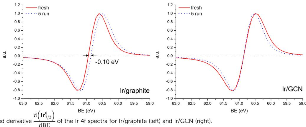
Fig. 8 Normalized derivative  $\frac{d(Ir_{7/2}^0)}{dBE}$  of the Ir 4f spectra for Ir/graphite (left) and Ir/GCN (right).
