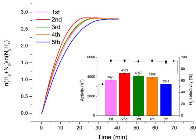
**Fig. 3** Stability tests for 1 wt% Ir/GCN. The insets are the catalytic activity (left axis) and H<sub>2</sub> selectivity (right axis) trends along repeated cycles. All tests were performed at 323 K and 1400 rpm, using 300  $\mu$ L of a 3.3 M hydrazine solution in 5 mL of 0.5 M NaOH and a N<sub>2</sub>H<sub>4</sub>· $\cdot$ -H<sub>2</sub>O: catalyst molar ratio of 1000:1. A sampling time of 0.3 s was employed to obtain continuous kinetic profiles.
