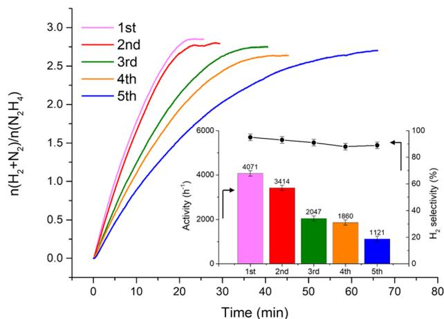
**Fig. 2** Stability tests for 1 wt% Ir/graphite. The insets are the catalytic activity (left axis) and  $\text{H}_2$  selectivity (right axis) trends along repeated cycles. All tests were performed at 323 K and 1400 rpm, using 300  $\mu\text{L}$  of a 3.3 M hydrazine solution in 5 mL of 0.5 M NaOH and a  $\text{N}_2\text{H}_4 \cdot \text{H}_2\text{O}$ : catalyst molar ratio of 1000 : 1. A sampling time of 0.3 s was employed to obtain continuous kinetic profiles.
