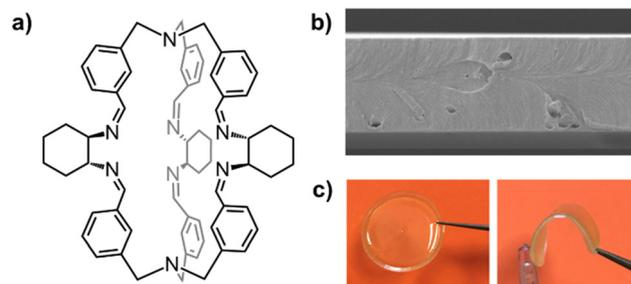
**Fig. 13** (a) Schematized structure of a chiral cage employed in the preparation of mechanically robust self-standing membranes with various thickness; (b) SEM image (25 K $\times$ ) of the cross-section of a thin membrane obtained from the neat cage (thickness: 4.3  $\mu\text{m}$ ); (c) pictures of a  $\sim 70$   $\mu\text{m}$  thick membrane of the same cage (20 mm diameter). Reproduced and adapted with permission from *Chem. – Eur. J.*, 2023, e202301437.<sup>105</sup>
