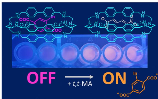
Fig. 3 Chemosensing device, based on  $[\text{Cu}_2(\mathbf{4})]^{4+}$  and 6-TAMRA (as selective host and fluorescent indicator, respectively), employed in the quantification of *t,t*-MA in spiked urine samples. Reproduced and adapted from *New J. Chem.*, 2018, **42**, 15460.<sup>56</sup>
