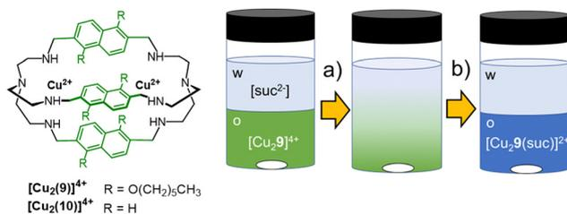
**Fig. 9** Schematized structures of the dicopper cryptates of cages **9** and **10**, and application of  $[\text{Cu}_2(\mathbf{9})]^{4+}$  as extractant for succinate<sup>76</sup> from aqueous solutions (0.05  $\text{mol L}^{-1}$  HEPES buffer, pH = 7) into dichloromethane. The transfer of succinate into the organic phase and its binding into the cryptate cavity are accompanied by a change of colour in the organic phase, from green to blue.
