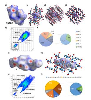
Fig. 4 (a) Hirshfeld surfaces. (b)–(d) close contacts. (e)–(f) Fingerprint plot and individual contacts.
