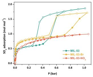
Fig. 2 Experimental SO<sub>2</sub> adsorption-desorption isotherms for fully activated MIL-53(Cr) (green), MIL-53(Cr)-Br (yellow), and MIL-53(Cr)-NO<sub>2</sub> (red) samples at 298 K and up to 1 bar. Filled circles = adsorption; open circles = desorption.
