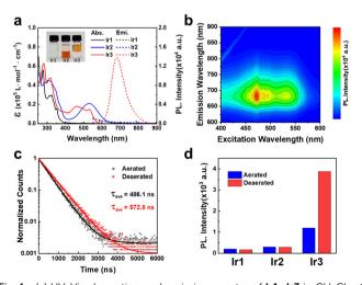
Fig. 1 (a) UV-Vis absorption and emission spectra of Ir1-Ir3 in  $CH_2Cl_2$  at room temperature. Insert:  $\log P_{\text{o/w}}$  of Ir1-Ir3 (b) 3D mapping phosphorescence spectra of the Ir3 (10  $\mu M$ ) in  $CH_2Cl_2$  at room temperature. (c) Phosphorescence lifetime of Ir3 in CH<sub>2</sub>Cl<sub>2</sub> under air or N<sub>2</sub>. (d) Phosphorescence intensity of Ir1-Ir3 (10 μM) in CH<sub>2</sub>Cl<sub>2</sub>.
