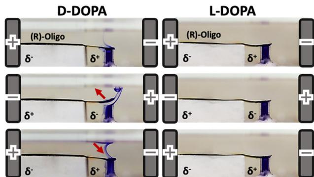
Fig. 8 Bipolar enantioselective valve operating with a Ppy actuator functionalized with (*R*)-oligo-BT<sub>2</sub>T<sub>4</sub> dipped in an aqueous 0.2 M LiClO<sub>4</sub> solution of 5 mM D-DOPA on the left and 5 mM L-DOPA on the right (Copyright © 2022, John Wiley and Sons).
