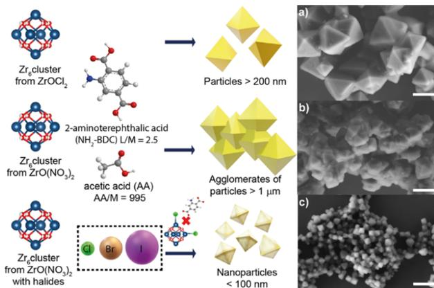
Fig. 4 Halide effect in the generation of UiO-66-NH<sub>2</sub> and UiO-66 nanocrystals (NMOFs). Representative micrographs of UiO-66-NH<sub>2</sub> produced using (a) ZrOCl<sub>2</sub> as a precursor without extra halides added, (b) ZrO(NO<sub>3</sub>)<sub>2</sub> as a precursor without extra halides added and (c) ZrO(NO<sub>3</sub>)<sub>2</sub> as a precursor with extra halides added. Scale bars correspond to 500 μm. Adapted with permission from ref. 33.
