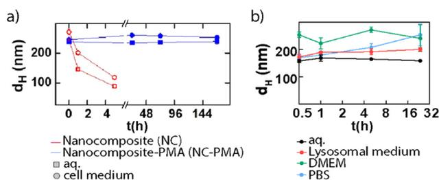
Fig. 12 Mean hydrodynamic diameter ( $d_h$ ) for (a) NMOF composites during one week (red) and NMOF composites-PMA (blue) systems in water and cell medium and (b) UiO-66-NH<sub>2</sub> NPs during 32 h in different media. Adapted with permission from ref. 14 and 33.
