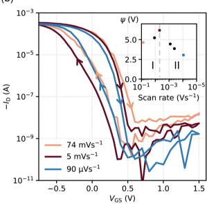
Fig. 4 (a) Transfer characteristics of different scan ranges ( $V_{GS,0}$  to  $V_{GS,1}$ ) revealed a saturation of the hysteresis ( $V_{\rm DS} = -0.1$  V). This behaviour is expressed through  $\psi$  parameters in the inset, normalized by  $\Delta(V_{GS})$  =  $V_{\rm GS,1}-V_{\rm GS,0}$ .  $V_{\rm GS,0}$  was fixed at -1.5 V. (b) The hysteresis changes with the scan rate, which can be divided into two regimes, as shown in the inset  $(V_{DS} = -0.1 \text{ V})$
