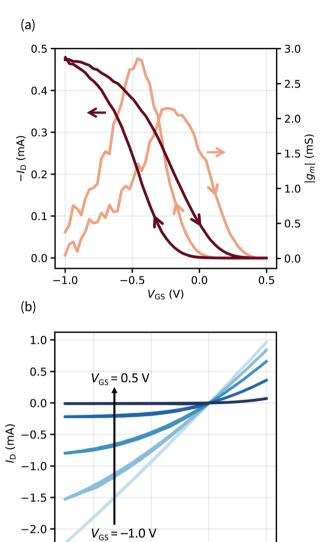
Fig. 2 (a) Transfer characteristic and transconductance ( $|g_m|$ ) of an OECT ( $V_{DS} = -0.1 \text{ V}$ ). (b) Output characteristics of the same device with  $V_{\rm GS} = -1.0 \text{ V}, -0.5 \text{ V}, -0.25 \text{ V}, 0 \text{ V}, \text{ and } 0.5 \text{ V}$
