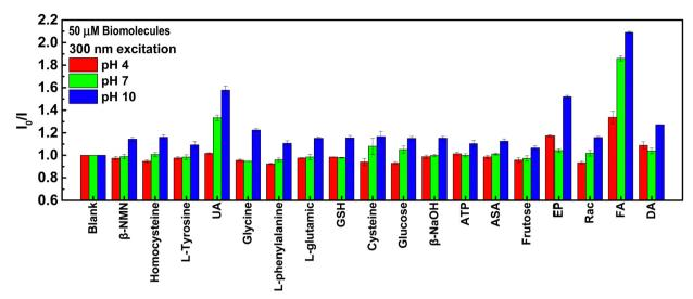
Selectivity test of biomolecules in various pH environments
