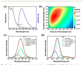
**Fig. 1** Spectroscopic characterization of NGQDs. (a) UV-Vis absorbance and PL emission spectra with the highest intensity. (b) PL map. XPS narrow scans on the (c) N 1s and (d) O 1s of NGQDs.
