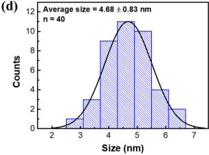
Fig. 2 TEM measurements of NGQDs. (a) Low magnification TEM, (b) FFT, (c) high magnification TEM images and (d) the corresponding particle size distribution of NGQDs.
