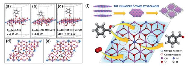
Fig. 22 DFT-calculated conformation of adsorption states and adsorption energies of a benzyl alcohol molecule on (a) an OV, (b) a  $V_{CO}$ -Co- $OH^{\delta-}$  site, and (c) defect-free Co-OH. Top views of the optimized structures of (d) an OV and (e) a Co vacancy. (f) Schematic diagram of Cocontaining LDH for the aerobic oxidation of alcohols. Reproduced with permission. Adapted with permission from ref. 182 Copyright (2018) American Chemical Society.
