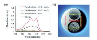
Fig. 4 (a) Detection of  $H_2O_2$  by activation of  $O_2$  over  $Mn_3O_4$  and Mn<sub>2</sub>O<sub>3</sub>, respectively. (b) Schematic illustration of the recycling strategy for  $\mbox{Mn}_3\mbox{O}_4$  and  $\mbox{Mn}_2\mbox{O}_3$  on  $\mbox{O}_2$  activation to generate  $\mbox{H}_2\mbox{O}_2$  that decomposes into HO\*. Adapted from ref. 120 with permission from The Royal Society of Chemistry.
