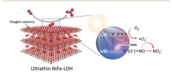
**Fig. 6** Schematic illustration of activation of  $O_2$  into  $O_2$  on NiFe-LDH with an OV for the selective photocatalytic oxidation of NO. Adapted with permission from ref. 140 Copyright (2022) American Chemical Society.
