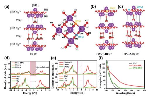
Fig. 8 The structural models of (a) BOC, (b) OVs1-BOC, and (c) OVs2-BOC, respectively. Contradistinction of DOS/PDOS (Fermi levels are set to 0 eV) between (d) BOC and OVs1-BOC and (e) BOC and OVs2-BOC. (f) Calculated optical absorption of BOC, OVs1-BOC, and OVs2-BOC. Adapted with permission from ref. 148 Copyright (2021) American Chemical Society.
