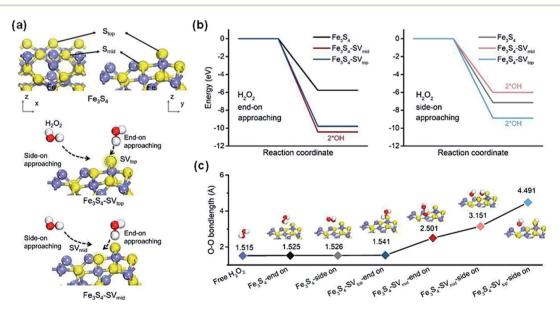
Fig. 2 (a) Models of  $Fe_3S_4$  and SVs-rich  $Fe_3S_4$  with exposure of the (011) surface. (b) Energy diagrams of  $H_2O_2$  adsorption on SVs-rich  $Fe_3S_4$  via end-on and side-on attachment models. (c) The O-O bond length of adsorbed  $H_2O_2$  in different adsorption configurations. Adapted with permission from ref. 110 Copyright (2021) Elsevier.
