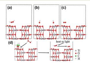
Fig. 5 Side view of (a) H<sub>2</sub>O<sub>2</sub> (b) initial configuration of two hydroxyl groups, and (c) superoxide radicals adsorbed on the TiO2 predicted by the GGA-TS method. (d) The decomposition mechanism of  $H_2O_2$  into superoxide radicals on TiO<sub>2</sub> NSs. Adapted with permission from ref. 132 Copyright (2017) American Chemical Society.
