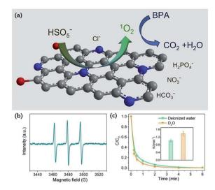
Fig. 18 (a) Schematic illustration of BPA degradation. (b) EPR spectrum of PMS activation. (c) Effect of D2O on BPA removal efficiency. Adapted with permission from ref. 275 Copyright (2019) Elsevier.
