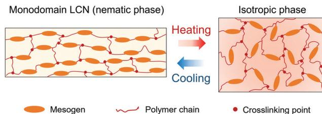
**Fig. 1** An illustration of the reversible shape changing mechanism in LCNs based on the transition between the nematic monodomain and isotropic states.
