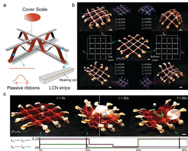
**Fig. 5** (a) Illustration of the layered soft robot including the cover scales, heating coil-embedded LCN strips, and passive Kapton ribbons. (b) Different attainable shapes of the robotic surface controlled by four independent current sources. (c) Robotic surface performing different tasks. Reproduced with permission.<sup>74</sup> Copyright 2021, AAAS.
