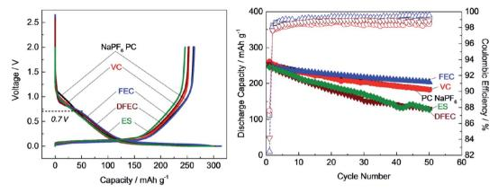
Fig. 3 Cycle performance of hard-carbon anode in 1 mol dm $^{-3}$  NaPF $_6$  in PC-based electrolyte containing 1 vol% of FEC, VC, ES and DFEC additives. Copyright 2016, John Wiley & Sons, Inc.
