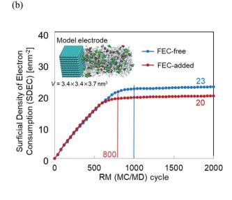
Fig. 5 (a) Charge/discharge curves (1<sup>st</sup> cycle, black line; 30<sup>th</sup> cycle, red line) of carbon-based electrode cycled<sup>23</sup> (Copyright 2016, John Wiley & Sons, Inc)., and (b) the electron consumption used for SEI film formation in NaPF<sub>6</sub> PC/FEC based electrolyte on carbon-based electrode.
