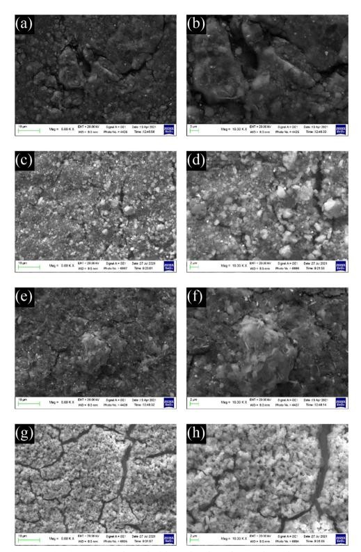
Fig. 7 SEM images of electrodes from formulations #1 (a and b), #2 (c and d), #3 (e and f), and #4 (g and h).
