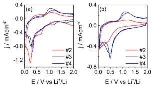
Fig. 8 1st CV (a) and 2nd (b) CV at 50  $\mu$ V s<sup>-1</sup> in LP30, WE: carbon electrodes, CE-RE: lithium, separator Whatman: GF/A
