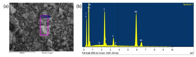
Fig. 2 SEM images of (a) pristine carbon ground in an agate mortar and (b) EDS analysis of the carbon ground in a mortar.
