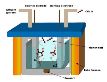
Fig. 1 Schematic of the MSCC-ET reactor.
