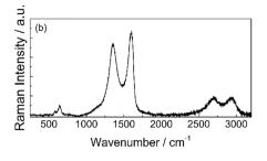
Fig. 4 (a) X-ray diffraction patterns of pristine synthesized carbon (red), C-50 (black) and diffractogram of Mn<sub>7.84</sub>O<sub>16</sub> (reference code 96-151-4117). (b) Raman spectrum of the carbon ground in an agate mortar.
