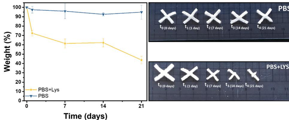
Fig. 7 Remaining weight in % after hydrolytic (PBS) and enzymatic (PBS + LYS) degradation and images of the aged samples.
