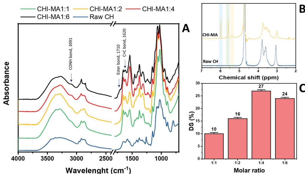
Fig. 2 FTIR spectra of raw chitosan and CHI-MA at different ratios of MA (A) and <sup>1</sup>H-NMR of CHI-MA (B). Degree of methacrylation of the samples prepared at different ratios of MA (C).
