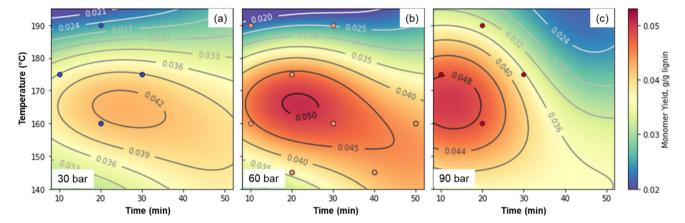
Fig. 8 Optimization of Sr(OH)<sub>2</sub>-promoted alkaline oxidation of DMR-EH lignin. (a). 30 bar total pressure. (b). 60 bar total pressure. (c). 90 bar total pressure. The machine learning fit used to generate the contour plots is shown in Fig. S10† and the numerical data corresponding to the monomer yields are provided in Table S11.†
