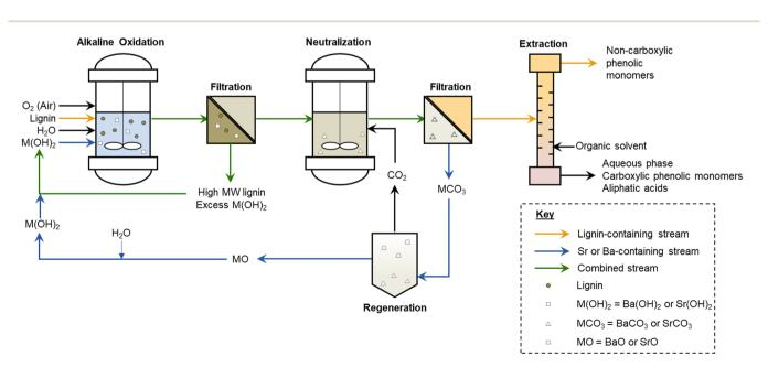
Fig. 1 Envisioned lignin upgrading process using reversibly-soluble alkaline earth metal hydroxides, such as Sr(OH)<sub>2</sub> and Ba(OH)<sub>2</sub>. This process is compared to other lignin upgrading strategies in Fig. S1.†
