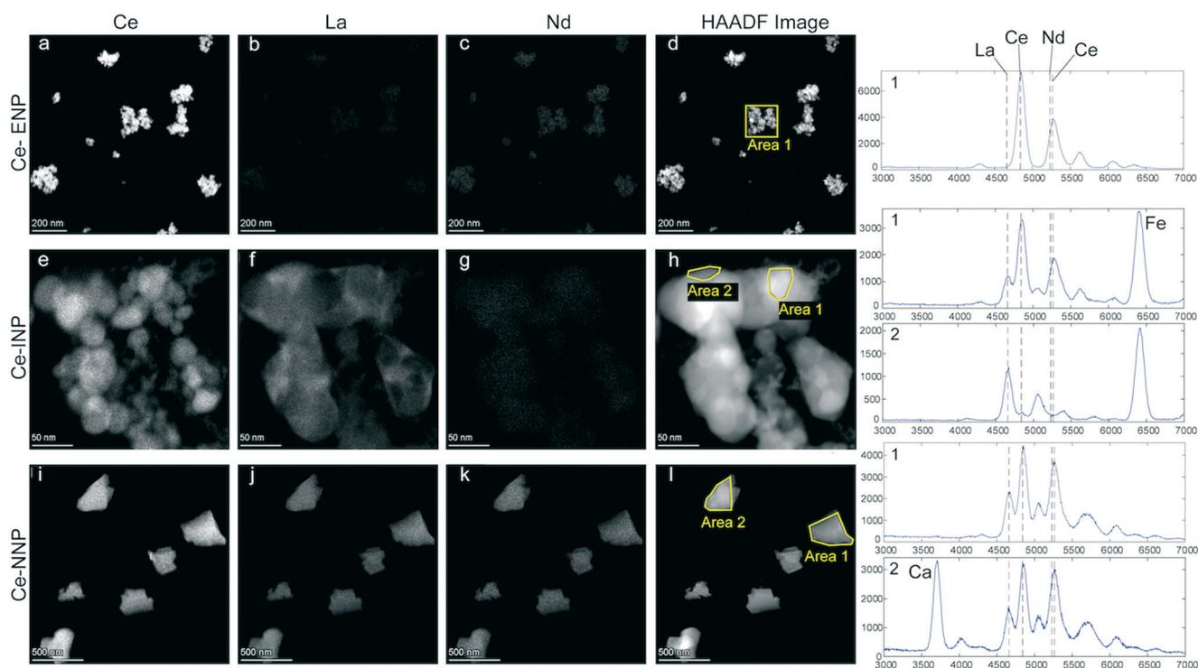
**Fig. 1** Elemental distribution maps of Ce, La, and Nd for  $\text{CeO}_2$  Ce-ENPs (a–c), ferrocerium lighter Ce-INPs (e–g), and bastnaesite/parisite Ce-NNPs (i–k). HAADF images (d, h and l) of the respective particle type show the morphology of individual particles. EDX spectra of the areas indicated are provided to the right of the images. The positions of the (main) X-ray lines for Ce, La, Nd, Ca, and Fe are labeled.
