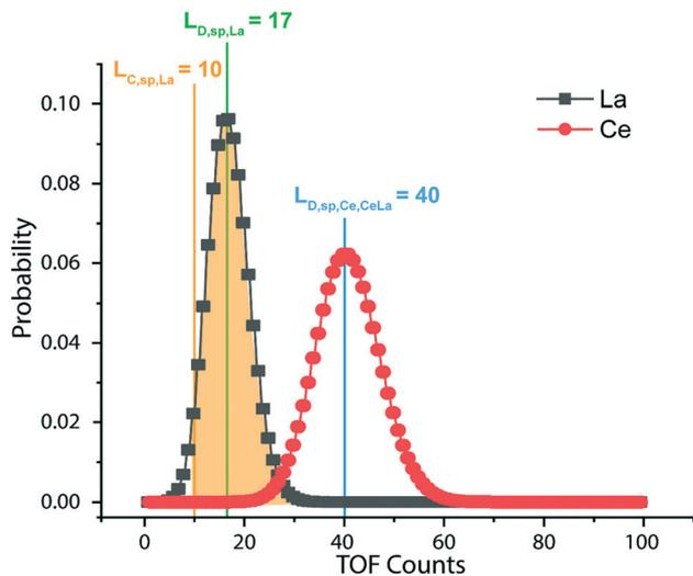
Fig. 6 Detection limits for mm-Ce-La NPs are a function of the critical value of La ( $L_{c,sp,La}$ ) as well as the ratio of Ce:La as controlled by Poisson statistics. Here, the detection limit for a Ce-La NP ( $L_{c,sp,Ce,Ce-La}$ ) is the average Ce signal that leads to 95% ( $\beta = 0.05$ ) of the La signal distribution to be above  $L_{c,sp,La}$ .
