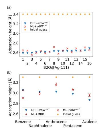
Fig. 6 (a) Adsorption heights of B2O molecules on Ag(111). (b) Adsorption heights of benzene, B2 naphthalene, B3 anthracene, B4 pentacene, B5 and azulene, B3 computed with ML+vdWsurf and compared to DFT+vdWsurf. The same adsorption sites as mentioned in the cited references (Table 1) are used.
