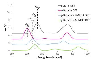
Fig. 3 Calculated INS spectra of unconfined antiperiplanar n-butane (Butane DFT) and gauche distorted butane unconfined (q-Butane DFT), within siliceous (Si-MOR) and acidic (Al-MOR) mordenite pores shows the deviation in the methyl torsion peak position between the conformers, akin to the experimental findings (Fig. 1). Spectra are artificially shifted by 1.5 (cm<sup>-1</sup>)<sup>-1</sup> for ease of reading.
