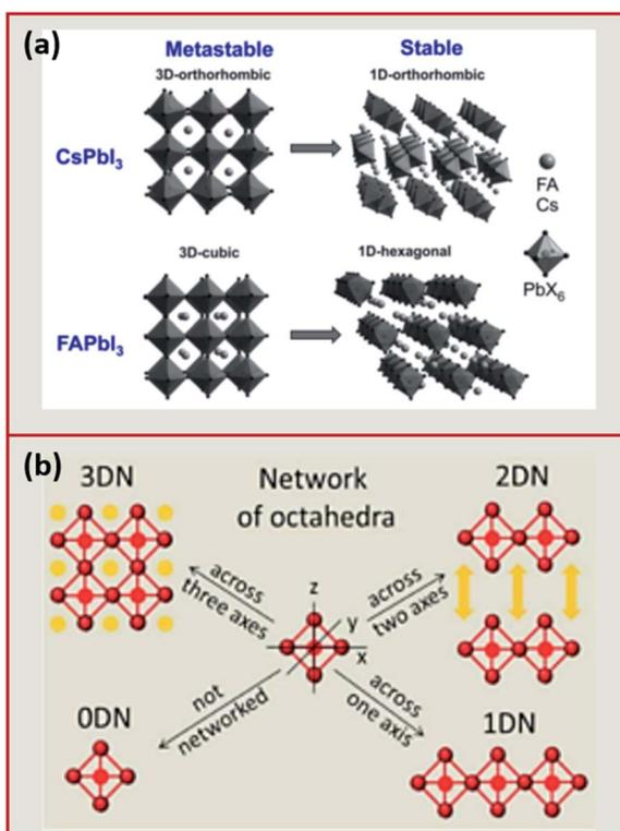
Fig. 2 (a) Illustration of the 3D to 1D phase transition in  $CsPbI_3$  and  $FAPbI_3$ . Reproduced with permission from ref. 27. (b) Schematic representing the differences between the different dimensionalities (ODN, 1DN, 2DN and 3DN) depending on the connectivity of the octahedra. Reproduced with permission from ref. 56.
