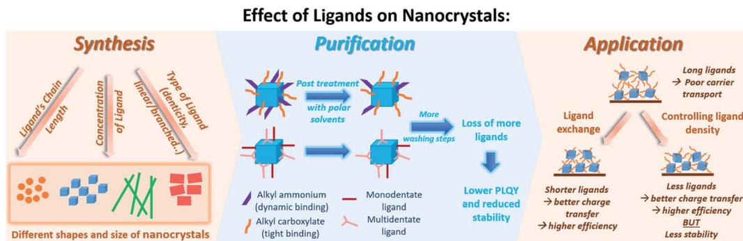
Fig. 20 A schematic showing the role of ligands during the synthesis, purification and application of perovskite NCs.
