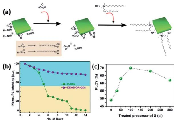
Fig. 16 (a) Illustration of the ligand exchange mechanism on CsPbBr<sub>3</sub> QDs. (b) The variation of PL intensity with respect to time for unmodified QDs and DDAB-OA treated QDs. Both (a) and (b) are taken with permission from ref. 199. (c) The variation of PLQY values of CsPbBr<sub>3</sub> QDs with the amount of the sulfide precursor added. This panel is taken with permission from ref. 200.
