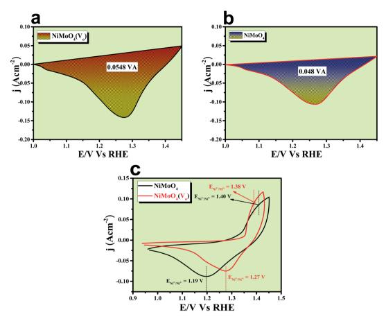
Fig. 11 (a) and (b) Reduction peak area of rod-like  $NiMoO_4(V_0)$  and  $NiMoO_4$ ; (c) CV cycles for  $NiMoO_4(V_0)$  and  $NiMoO_4$ .
