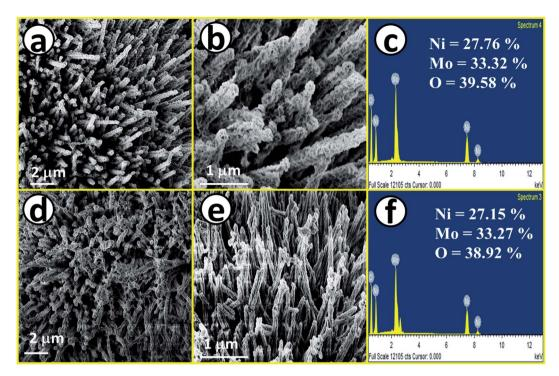
Fig. 2 (a) and (b) FE-SEM images of NiMoO<sub>4</sub> nano-rods, (c) EDS spectrum of NiMoO<sub>4</sub> in the FE-SEM mode, (d) and (e) FE-SEM images of NiMoO<sub>4</sub>( $V_o$ ) nanorod and (f) EDS spectrum of NiMoO<sub>4</sub>( $V_o$ ) in the FE-SEM mode.
