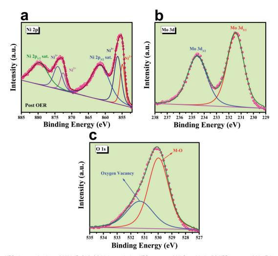
Fig. 12 Post XPS characterization of NiMoO<sub>4</sub>( $V_o$ ): (a) high-resolution XPS spectra of Ni 2p orbitals, (b) XPS spectra of Mo 3d orbital and (c) deconvoluted XPS spectrum of O 1s orbitals
