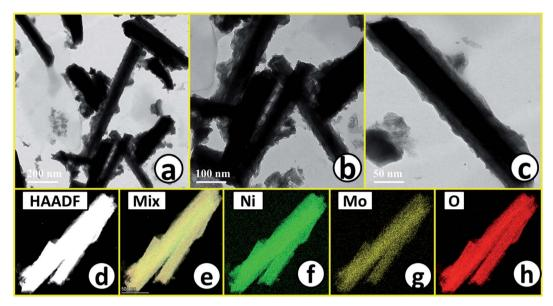
Fig. 4 (a)–(c) Low to high magnification HR-TEM images of NiMoO<sub>4</sub>( $V_o$ ); (d) is the HAADF image of rod-like NiMoO<sub>4</sub>( $V_o$ ) taken for the mapping analysis; (e)-(h) are the characteristic mapping results of mix, Ni K, Mo K, O K and respectively.
