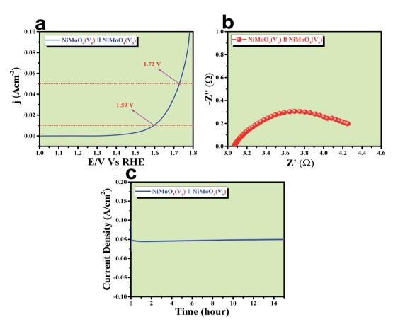
Fig. 10 (a) LSV curve of rod like NiMoO<sub>4</sub>( $V_o$ ) as an anode and cathode in a two electrode system at a scan rate of 2 mV s<sup>-1</sup>, (b) impedance spectra obtained at 400 mV overpotential, and (c) chronoamperometric outcomes for 15 hours.
