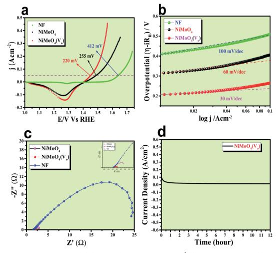
Fig. 7 (a) Is the backward CV of rod like  $NiMoO_4(V_0)$  and  $NiMoO_4$  at a scan rate of 5 mV s<sup>-1</sup>, (b) corresponding Tafel plot, (c) impedance spectra obtained at 300 mV overpotential and (d) chronoamperometric outcomes for 12 h.
