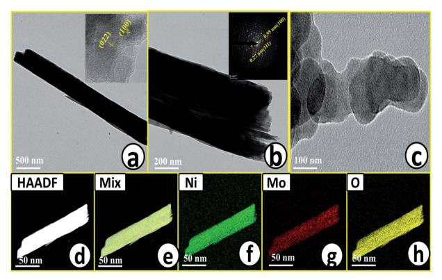
Fig. 3 (a) and (c) Low to high magnification HR-TEM images of NiMoO<sub>4</sub>, inset of (a) and (b) are corresponding lattice fringes and SAED pattern respectively, (d) is the HAADF image of rod-like NiMoO<sub>4</sub> taken for the mapping analysis, (e)–(h) are the characteristic colour mapping results of mix, Ni K, Mo K and O K respectively.
