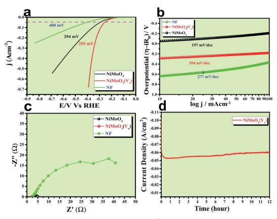
Fig. 9 (a) LSV curve of rod like NiMoO<sub>4</sub>(V<sub>o</sub>) and NiMoO<sub>4</sub> at a scan rate of 5 mV s<sup>-1</sup>, (b) corresponding Tafel plot, (c) impedance spectra obtained at 250 mV overpotential and (d) chronoamperometric outcomes for 12 hours
