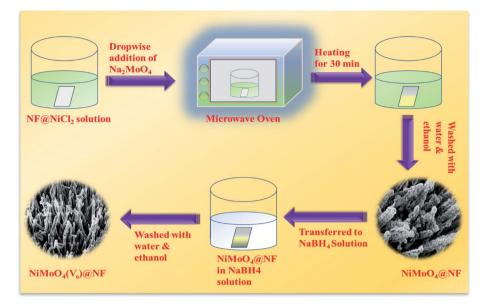
Scheme 1 A synthetic scheme for synthesizing NiMoO<sub>4</sub> and NiMoO<sub>4</sub>(V<sub>o</sub>) via a microwave heating method.
