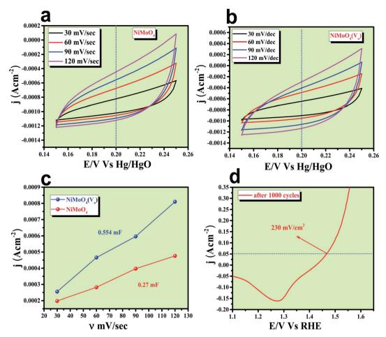
Fig. 8 (a) and (b) Are the CVs recorded for NiMoO<sub>4</sub> and NiMoO<sub>4</sub>( $V_0$ ) respectively in a non-faradaic region with increasing scan rate for the determination of ECSA from its double layer capacitance; (c) are the corresponding plots to the measure  $C_{al}$ ; (d) backward CV after 1000 cycles of AD study.
