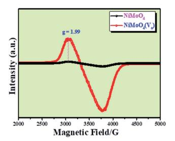
Fig. 6 EPR spectra of NiMoO<sub>4</sub> and NiMoO<sub>4</sub>(V<sub>o</sub>) at room temperature.
