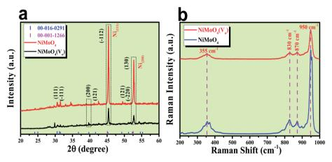
Fig. 1 (a) XRD patterns of rod shaped NiMoO<sub>4</sub> and NiMoO<sub>4</sub>( $V_0$ ), (b) Raman spectra of rod shaped NiMoO<sub>4</sub> and NiMoO<sub>4</sub>( $V_0$ ).
