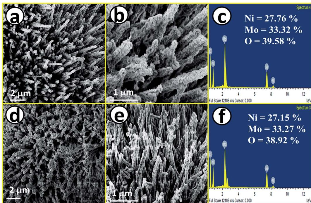
Fig. 2 (a) and (b) FE-SEM images of  $\text{NiMoO}_4$  nano-rods, (c) EDS spectrum of  $\text{NiMoO}_4$  in the FE-SEM mode, (d) and (e) FE-SEM images of  $\text{NiMoO}_4(\text{V}_o)$  nanorod and (f) EDS spectrum of  $\text{NiMoO}_4(\text{V}_o)$  in the FE-SEM mode.
