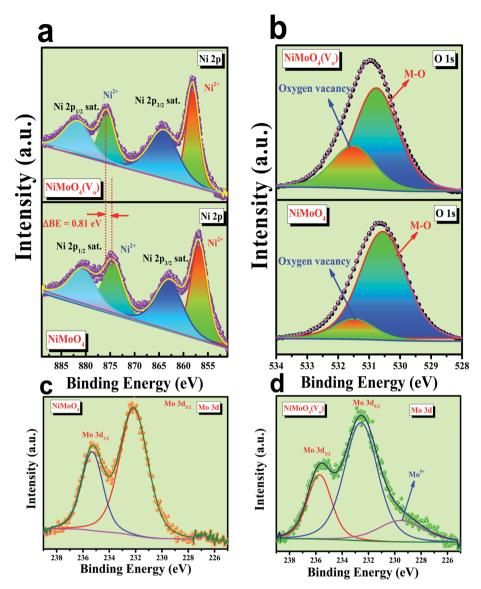
Fig. 5 (a) Combined high-resolution XPS spectra of Ni 2p orbitals for NiMoO<sub>4</sub> and NiMoO<sub>4</sub>( $V_o$ ), (b) deconvoluted XPS spectrum of O 1s orbitals, (c) XPS spectra of Mo 3d orbital of NiMoO<sub>4</sub> and, (d) XPS spectra of Mo 3d orbital of NiMoO<sub>4</sub>( $V_o$ ).
