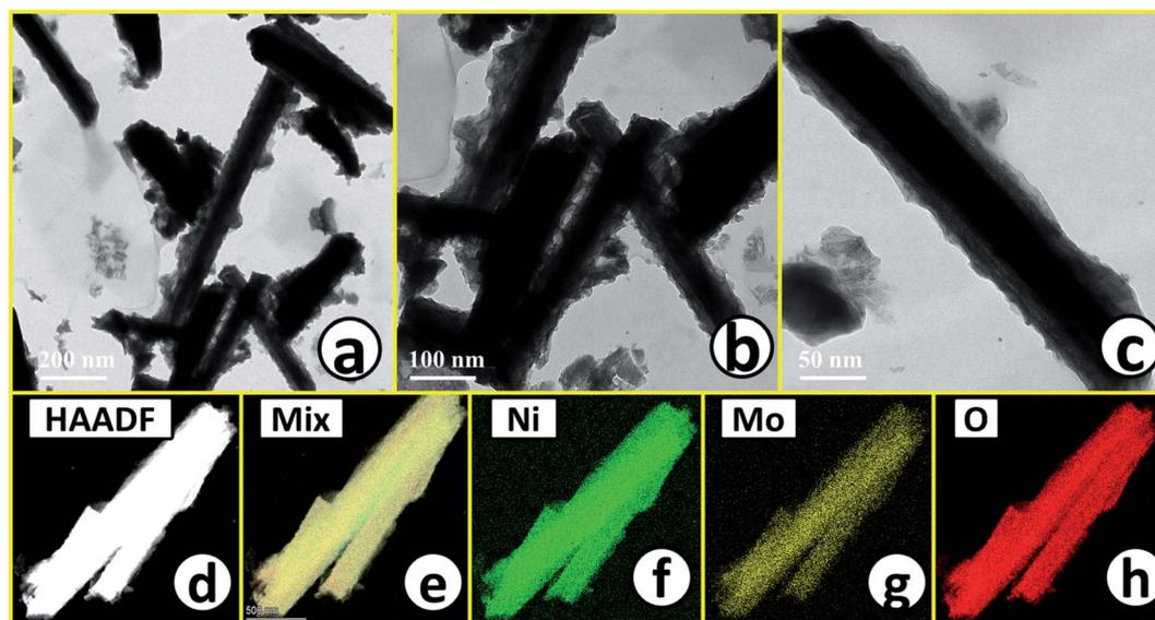
Fig. 4 (a)–(c) Low to high magnification HR-TEM images of  $\text{NiMoO}_4(\text{V}_\text{o})$ ; (d) is the HAADF image of rod-like  $\text{NiMoO}_4(\text{V}_\text{o})$  taken for the mapping analysis; (e)–(h) are the characteristic mapping results of mix, Ni K, Mo K, O K and respectively.
