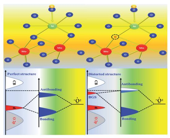
Scheme 3 Schematic representation of molecular orbital and band structure, for the origination of high electrocatalytic activity of NiMoO<sub>4</sub>(V<sub>o</sub>) through vacancy formation.
