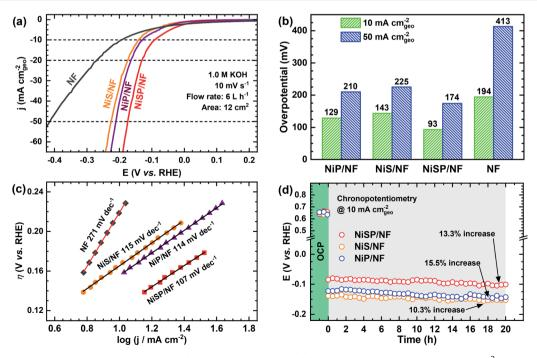
Fig. 5 HER electrochemical characterization results: (a) cathodic i-V curves, (b) overpotentials at 10 and 50 mA cm<sup>-2</sup>, (c) Tafel slopes, and (d) chronopotentiometric runs at 10 mA cm<sup>-2</sup> for 20 h using the as-prepared electrodes in 1 M KOH electrolyte.
