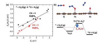
Fig. 5 (a) Shifted linear scaling relationships between  $E_{\rm f}$  and  $E_{\rm a}(N_2{\rm O})$  determined by CN. Black and red data points represent M@N $_3$  and M@N $_4$ , respectively. (b) The optimized geometries of the IS, TS and FS for \*O formation when using N $_2{\rm O}$  and associated energy diagram for  $E_{\rm a}(N_2{\rm O})$ .  $E_{\rm a}(N_2{\rm O})$  < 0 eV indicates that \*O formation proceeds via exothermic N $_2{\rm O}$  adsorption and low activation energy.
