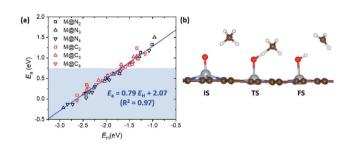
Fig. 4 (a) Linear scaling relationship between  $E_{\rm H}$  and  $E_{\rm a}$ . The area shaded in blue is  $E_{\rm a}$  < 0.75 eV. (b) The optimized geometries for the initial state (IS), transition state (TS) and final state (FS) in methane activation.
