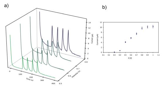
Fig. 4 Effect of the oxidation potential applied on the analytical response vs. Ag reference electrode (LMG concentration used was 1.0 mM in 50 mM ammonium acetate buffer pH =  $4.0 \pm 0.02$  with ACN (40% v/v) and Tween-80 (1% v/v)). (a) Amperometric determination of LMG on the  $\mu$ FIA system using different oxidation potentials (0.5–0.8 V). (b) Hydrodynamic voltammetry I-E curve obtained for a 3  $\mu$ L injection of LMG solution.
