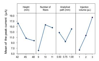
Fig. 5 Effect of the control factors on the mean peak current obtained. Optimal conditions are height of the device: 42 mm, number of fibers: 10, analytical path: 1.00 cm and injection volume: 3  $\mu$ L. All the measurements were performed in triplicate.
