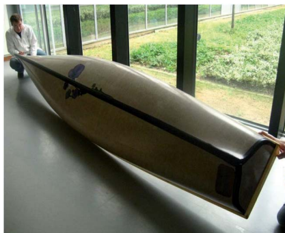
Fig. 2 Flax/PLA canoe manufactured during the NAVECOMAT project.
