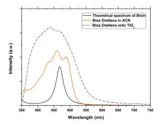
Fig. 4 Experimental absorption spectra of the dye obtained from Bixa orellana in solution and adhered to  $TiO_2$  compared with the theoretical spectrum obtained for bixin.
