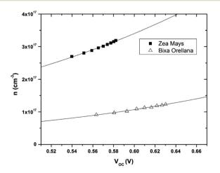
Fig. 9 Electronic density extracted as a function of open circuit voltage with its corresponding adjustment curves according to egn (3).
