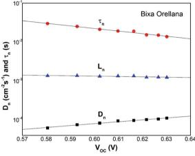
**Fig. 14** Diffusion length of the solar cell calculated from the electron lifetime and the chemical diffusion coefficient.
