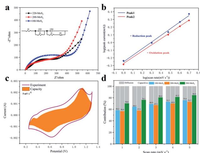
Fig. 7 (a) Electrochemical impedance spectroscopy of MoS<sub>2</sub> at different temperatures (inset is the equivalent circuit for fittings of the Nyquist plots of MoS<sub>2</sub>), (b)  $\log(i)$  and  $\log(v)$  curves of two peaks corresponding to the CV curves (200-MoS<sub>2</sub>), (c) capacitive contribution (orange) of 5 mV s<sup>-1</sup>, (d) capacitive and diffusion-controlled contribution ratios at multiple scan rates of MoS<sub>2</sub>.
