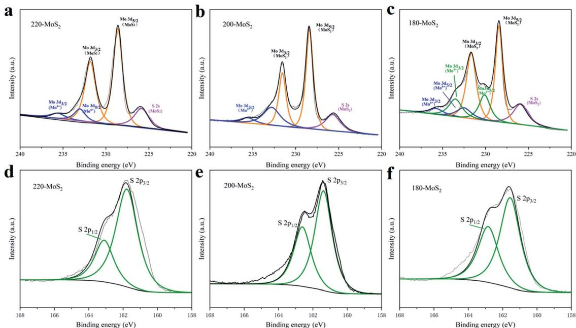
Fig. 5 (a–c) Mo 3d and (d–f) S 2s high-resolution XPS spectra of MoS<sub>2</sub> prepared at different temperatures.
