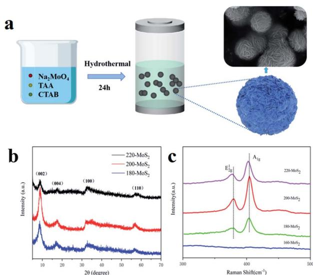
Fig. 1 (a) Schematic illustration of the preparation process of MoS<sub>2</sub>, (b) XRD of MoS<sub>2</sub> synthesized at different temperatures, (c) Raman spectra of MoS<sub>2</sub> synthesized at different temperatures.
