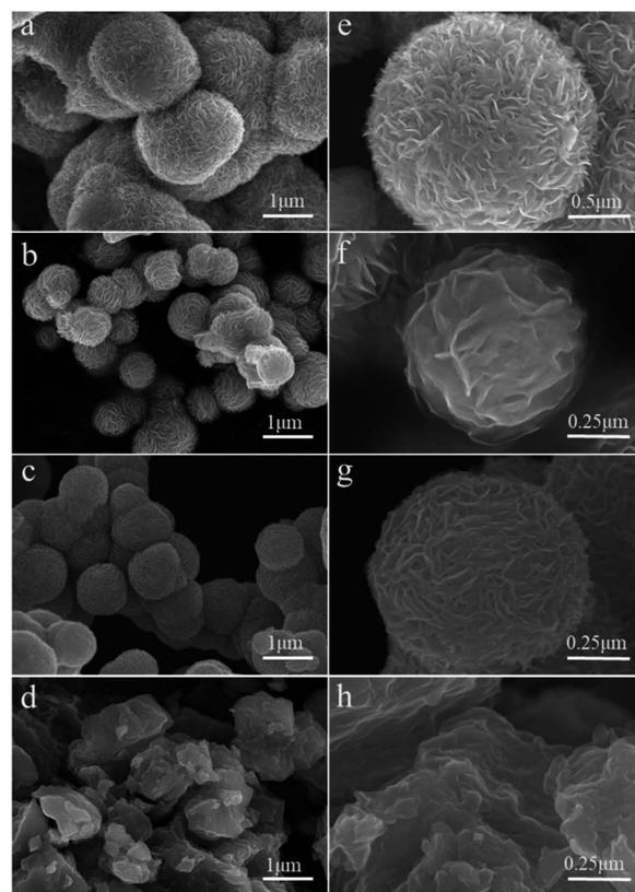
Fig. 2 (a and e) SEM images of 220-MoS<sub>2</sub>, (b and f) SEM images of 200-MoS<sub>2</sub>, (c and g) SEM images of 180-MoS<sub>2</sub>, (d and h) SEM images of 160-MoS<sub>2</sub>.
