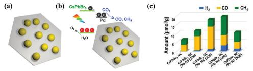
Fig. 15 (a) Diagram of the CsPbBr<sub>3</sub> NC/Pd-NC composite. (b) The sketch of the composite materials (CsPbBr<sub>3</sub> NC)/(Pd-NC) and their band alignments. (c) Photocatalytic CO<sub>2</sub> reduction performance. (a-c) Reprinted (adapted) with permission from ref. 100, Copyright 2018 American Chemical Society.
