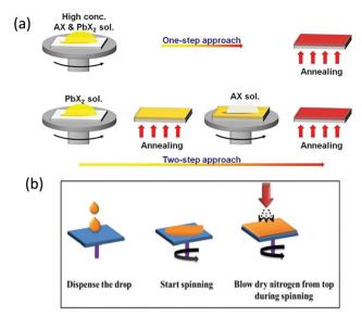
Fig. 6 Representation of one-step and two-step strategies for the preparation of perovskite films. AX and  $PbX_2$  symbolize CsBr and  $PbBr_2$ , respectively. Reprinted with permission ref. 106. Copyright 2019, The Royal Society of Chemistry. (b)  $N_2$  gas flow-assisted method for the fabrication of pinhole-free CsPbBr $_3$  thin films. Reprinted from ref. 119. Copyright 2020, Gupta, Kulbak, and Cahen.
