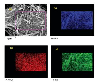
Fig. 4 FESEM (a) and elemental maps of (b) Mn; (c) C, and (d) O for  $0La-MnO_2-CNT$ .
