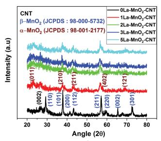
Fig. 1 XRD pattern of undoped and La<sup>3+</sup>:MnO<sub>2</sub>-CNT nanohybrid.
