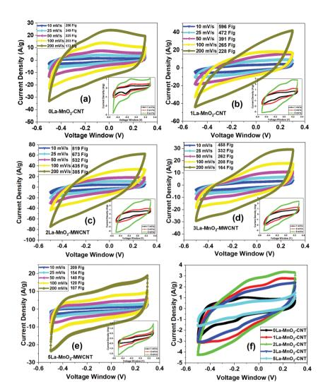
Fig. 7 CV curves of  $0La-MnO_2-CNT$  (a) and various La doped  $MnO_2-CNT$  hybrids (b-e) at varying scan rates; (insets of (a-e) show the curves at low scan rates); (f) comparative CV curves of all the samples at 5 mV s<sup>-1</sup> scan rate.
