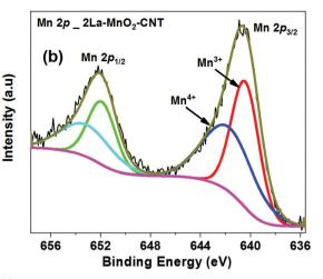
Fig. 3 XPS spectra of Mn 2p of OLa-MnO<sub>2</sub>-CNT (a) and 2La-MnO<sub>2</sub>-CNT (b).
