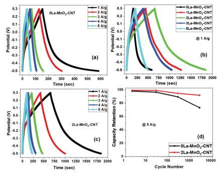
Fig. 9 GCD profiles of  $0La-MnO_2-CNT$  at different constant current densities (a); comparative GCD profiles of undoped and  $La^{3+}$   $MnO_2-CNT$  nanohybrids at 1 A  $g^{-1}$  (b); GCD profiles of  $2La-MnO_2-CNT$  at 1 A  $g^{-1}$  (c); cycle stability of  $0La-MnO_2-CNT$  and  $2La-MnO_2-CNT$  at 5 A  $g^{-1}$  up to 5000 cycles (d).
