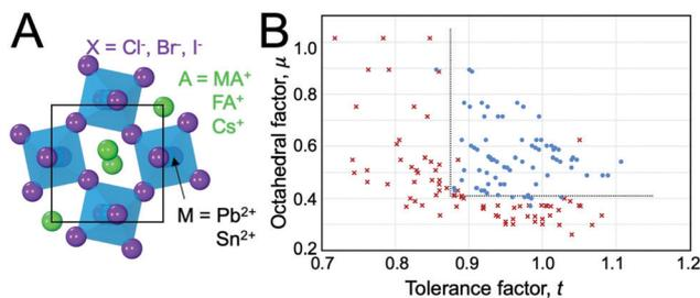
**Fig. 1** (A) Perovskite structure comprising corner-sharing octahedra. (B) Plot of octahedral factors *versus* tolerance factors based on anion-dependent cationic radii. Blue circles represent compounds that form the perovskite structure at room temperature and pressure, while red 'x's represent those that do not. Adapted from ref. 15. Copyright 2016, Royal Society of Chemistry.
