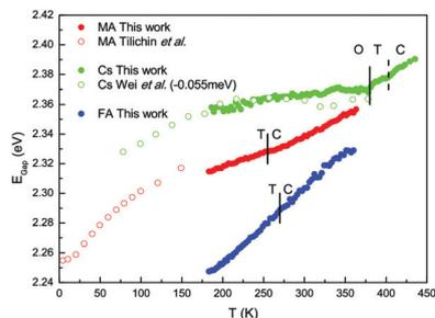
Fig. 12 Comparison of optical bandgap of MAPbBr<sub>3</sub>, CsPbBr<sub>3</sub>, and FAPbBr<sub>3</sub> single crystals. Cubic, tetragonal and orthorhombic phases are indicated by C, T, and O labels, respectively. Reproduced with permission from ref. 184. Copyright 2020, American Chemical Society.
