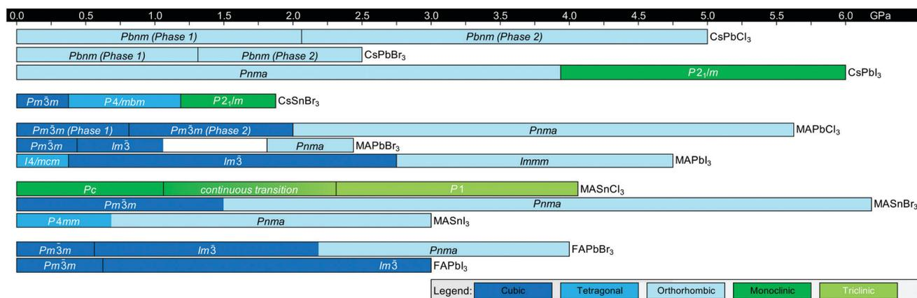
Fig. 11 Summary of room-temperature phase transition pressures in halide perovskites as a function of composition reported in the literature.<sup>162–170</sup> The white section in the data for  $\text{MAPbBr}_3$  indicates a region where data was not available.
