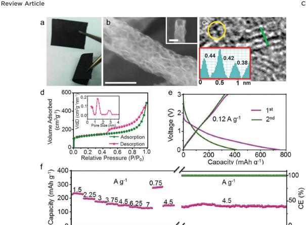
Fig. 18 (a) Digital photograph, (b) SEM image (scale bars: 100 nm), (c) high-resolution TEM image, (d) nitrogen adsorption-desorption isotherms and pore-size distributions, (e) charge-discharge voltage profiles at 0.12 A g<sup>-1</sup>, and (f) cycling performance at 4.5 A g<sup>-1</sup> of the polyacrylonitrile/Zn(Ac)<sub>2</sub>/Co(Ac)<sub>2</sub> nanofiber derived porous carbon nanofiber networks. Reproduced from ref. 331 with permission from Elsevier.
