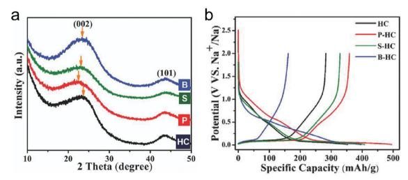
Fig. 19 (a) XRD patterns of doped and undoped carbons. After P- and S-doping, the (002) peak shifts to a lower angle, which indicates a larger d-spacing. However, B-doping barely shifts the peak. (b) Galvanostatic sodiation/desodiation potential profiles of hard carbon and doped hard carbons at a current rate of 20 mA  $g^{-1}$ . Reproduced from ref. 339 with permission from Wiley-VCH.
