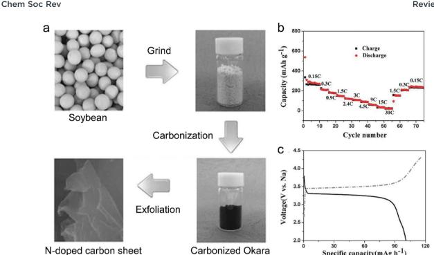
Fig. 17 (a) Schematic representation of the preparation of N-doped carbon sheets. (b) The capacity retention of the N-doped carbon sheets at current densities from 56.25 mA  $g^{-1}$  to 11.25 A  $g^{-1}$ . (c) Charge and discharge curves of the carbon sheets//Na<sub>3</sub>V<sub>2</sub>(PO<sub>4</sub>)<sub>3</sub> sodium ion batteries at 562 mA  $g^{-1}$ . Reproduced from ref. 316 with permission from Wiley-VCH.
