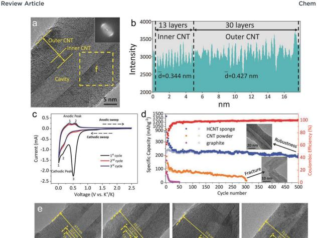
Fig. 20 (a) TEM image of a CNT. (b) Line profile obtained from the wall of a CNT. (c) CV curves of CNT sponge at  $0.3 \text{ mV s}^{-1}$ . (d) Cycling performance of CNT sponge, commercial CNT powder and graphite electrodes at a current density of 100 mA  $g^{-1}$ . (e) Ex situ TEM images of the CNT structure at different potassiation and de-potassiation potential in the first cycle. Reproduced from ref. 344 with permission from Wiley-VCH.
