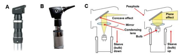
Fig. 3 Different types of retinoscopes and working scheme. (A) Streak retinoscopes: the light source produces a line or streak of light. (B) Spot retinoscope: the light source produces a spot of light. (C) Operating principles: both streak and spot retinoscopes have similar working principles, and the light can be adjusted by moving the sleeve to achieve a concave or plane effect. Copyright 2017, Community Eye Health.
