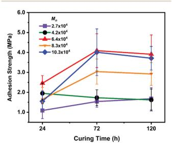
Fig. 1 Adhesion strength with different curing times. Error bars indicate standard deviation,  $n \ge 5$ .
