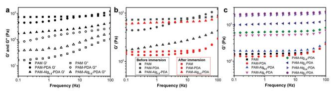
Fig. 5 The dynamic rheological behavior of various hydrogels. (a) The storage modulus (G') and loss modulus (G'') of hydrogels before immersion in artificial seawater; (b) comparison of G' of hydrogels before and after immersion in seawater for 3 days; (c) the change in G' of hydrogels with the concentration of Alg-Na immersed in artificial seawater for 3 days.
