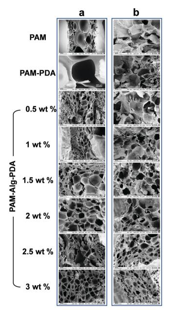
Fig. 2 SEM morphology images of cross sections of PAM-Alg-PDA hydrogel with different concentrations of Alg-Na, PAM-PDA hydrogel and PAM hydrogel (a) before immersion in artificial seawater and (b) after immersion in artificial seawater for 3 days
