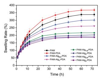
Fig. 4 The swelling behavior of various hydrogels
