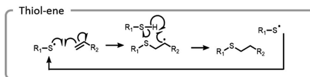
Fig. 12 Mechanism of thiol-ene catalytic reaction.
