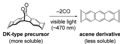
Fig. 1 Formation of acene derivatives via light-induced decarbonylative aromatization of DK-type photoprecursors.
