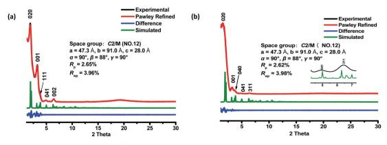
Fig. 2 PXRD patterns of COF-1 (a) and COF-2 (b) after Pawley refinement. PXRD profiles of the experimental pattern (black curve), Pawley refined (red curve), and calculated (green curve) patterns from the two-fold interpenetrated ffc modeled structure; their difference (blue curve).
