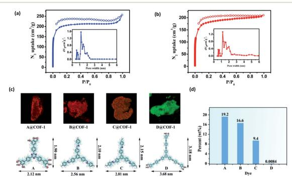
Fig. 4 (a)  $N_2$  adsorption—desorption isotherms (77 K) and pore size distribution profiles of COF-1; (b)  $N_2$  adsorption—desorption isotherms (77 K) and pore size distribution profiles of COF-2. (c) CFM images obtained from COF-1 after incubation with dyes A-D, respectively. (d) Different dye uptake released from COF-1 by UV-vis spectroscopy.
