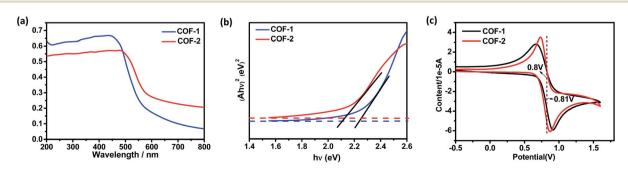
Fig. 5 (a) Solid-state UV spectra of the COFs. (b) Tauc plot for absorption spectra obtained with the Kubelka–Munk function and the linear fit for direct band gaps of the COFs. (c) Solid-state CV of the COFs with a scan rate of 50 mV s $^{-1}$ .
